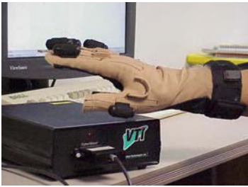
Fig. 1. Cyberglove™ with 18 sensors
